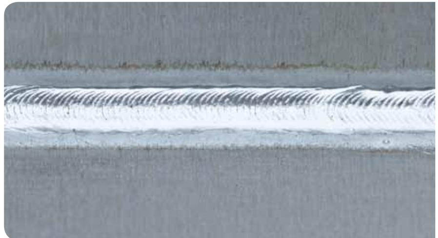
*Weld seam – e.g. Cold Weld process*
