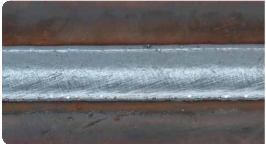
*Weld seam – e.g. Speed Weld process*
